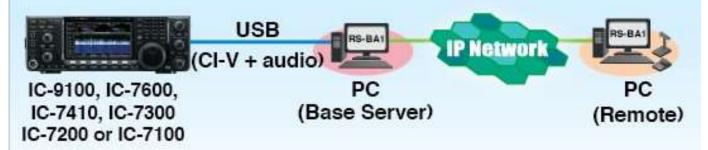
Some models (7800, 7610) direct to IP Network without Base Server. But Base Server useful to control other shack functions (rotators, amplifier,...)
