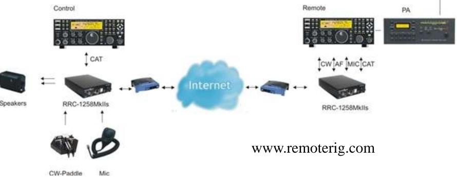
Use a pair of RemoteRig "modems" to send audio and control signals to station. Can use with: detached front panel (TS-480), "control heads" (Elecraft K3/0-Mini), "twin" radios, a PC program or an Android App.
