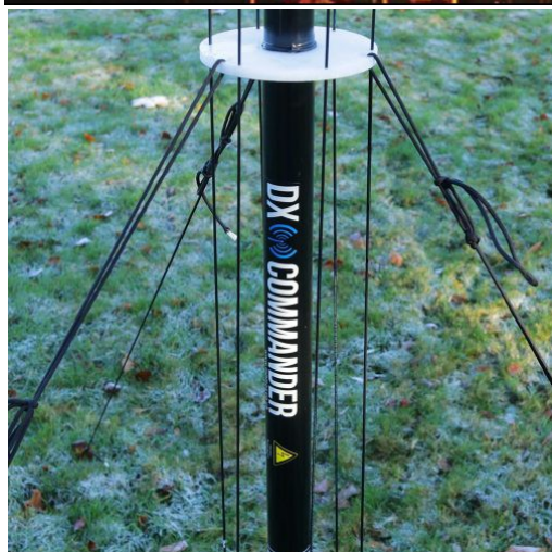
Fig 1, Base of DX Commander with radials. Note multiple radials
