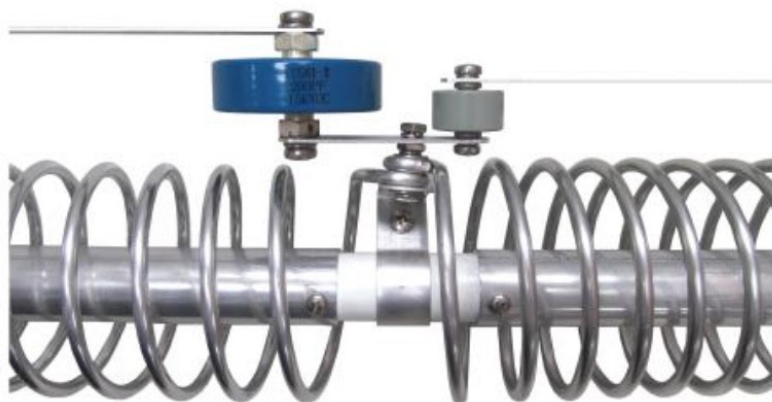
Fig 2. Closeup of a Butternut trap. This is a very robust and low-loss design.
