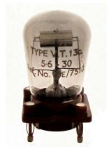
The VT13c is a 30-watt triode with a mu of 35. The filament uses 5.6 volts at 1.45 amps and up to 1500 volts on the plate. The maximum frequency is 6 MHz. The first
