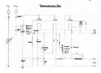
[Ed. Note: Norm also supplied a schematic of the RAF TR2 CW, ICW, and AM transmitter using 3 VT13C tubes. It's sort of quaint, probably hand drawn by a draftsman. You may want to study it carefully, a part of it will be reprised in this issue]
