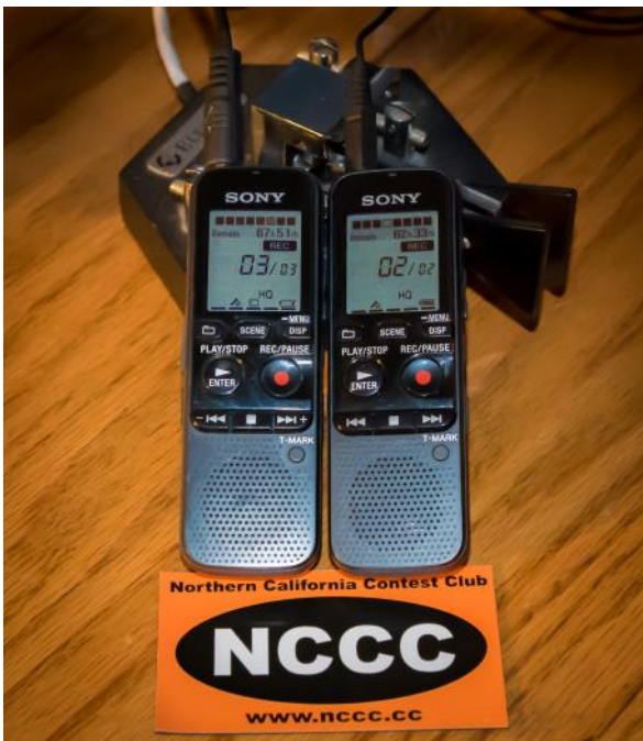
Figure 1. Sony ICD-PX333 Digital Voice Recorder. 2GB version with 4GB microSD card installed (left). 4GB (right). See the difference? Neither do I.
