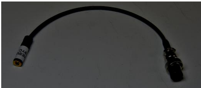
Fig 3 – Adapter For Computer Mic to Yaesu FT1000MP
