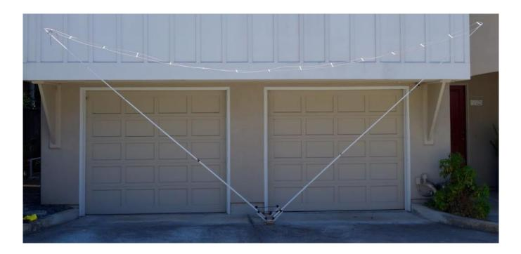
Here is 1 element of my antenna with the wire attached. The sag was roughly 2.5 feet, which is greater than the 1.4 or so feet calculated. The difference is due to the deflection of the tubing under the tension of the wire.
