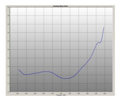
Of course SWR isn't the only measure of antenna performance – the coaxial resonator presents a low Q LC circuit and has a loss of about 1 dB at the band edges with much lower loss in between.
