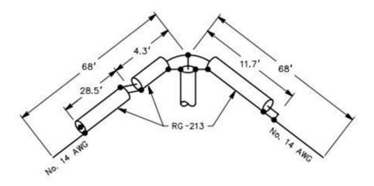
This antenna uses a Coaxial Resonator to broadband an 80m dipole. I found the original description in the QST archives – if you are an ARRL member you can access the article by searching for:
