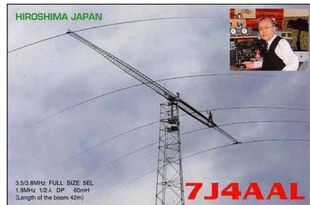
A full-size, 5 element, 80 meter yagi (Drool).
