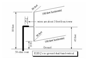
You'll note that Toman's antenna is a dual-band affair for both 80 and 160. Mine is a derivation for just 160. Also, his antenna made use of an 80-foot tower. My tower is just 72 feet, so my vertical section is almost 10 feet shorter and my horizontal sections are a little bit longer. However, like Toman's antenna, the bottom horizontal section is 10 feet off the ground, and the horizontal sections are parallel to one another in a vertical plane.
