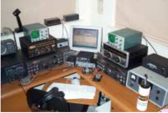
Today's SO2R set up – FT 1000s on right and left, Alpha 87A for left radio, Collins for right radio. DX Doubler switcher and ICE 419A bandpass filters.
