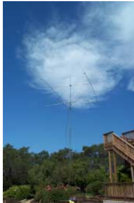
The main antennas are a Force 12 C31-XR at 50 feet and a MAG 240 N at 60 feet. Not visible are the half slopers for 80 and 160.
