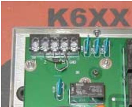
**Photo 2. View of diodes needed inside the StackMatch for the single-wire two-stack controller.**
