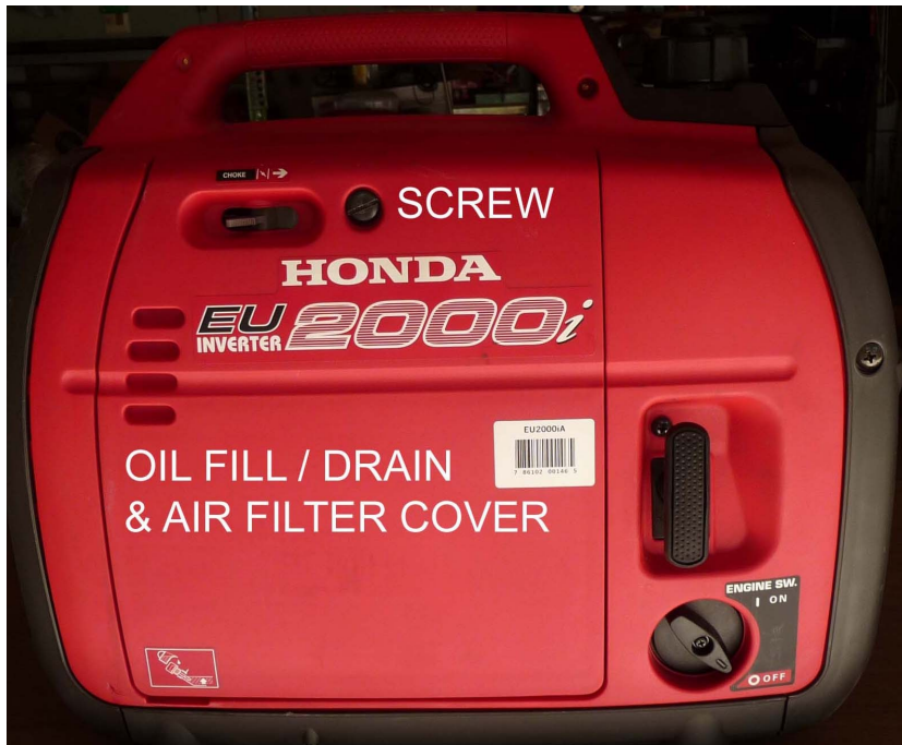
Figure 4. Oil fill / drain & air filter cover
