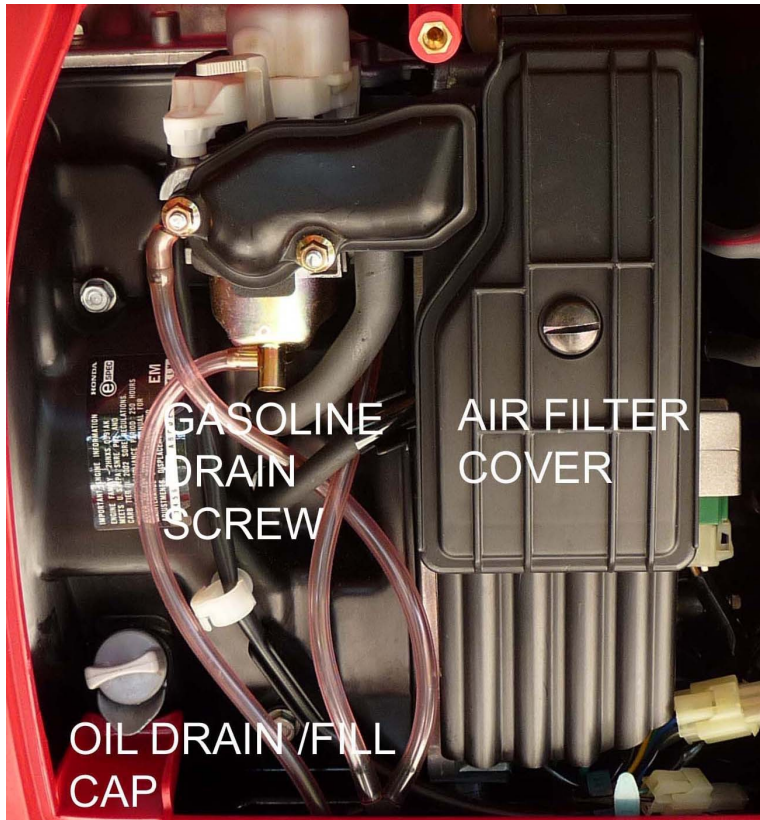
Figure 5. Location of oil cap and air filter
