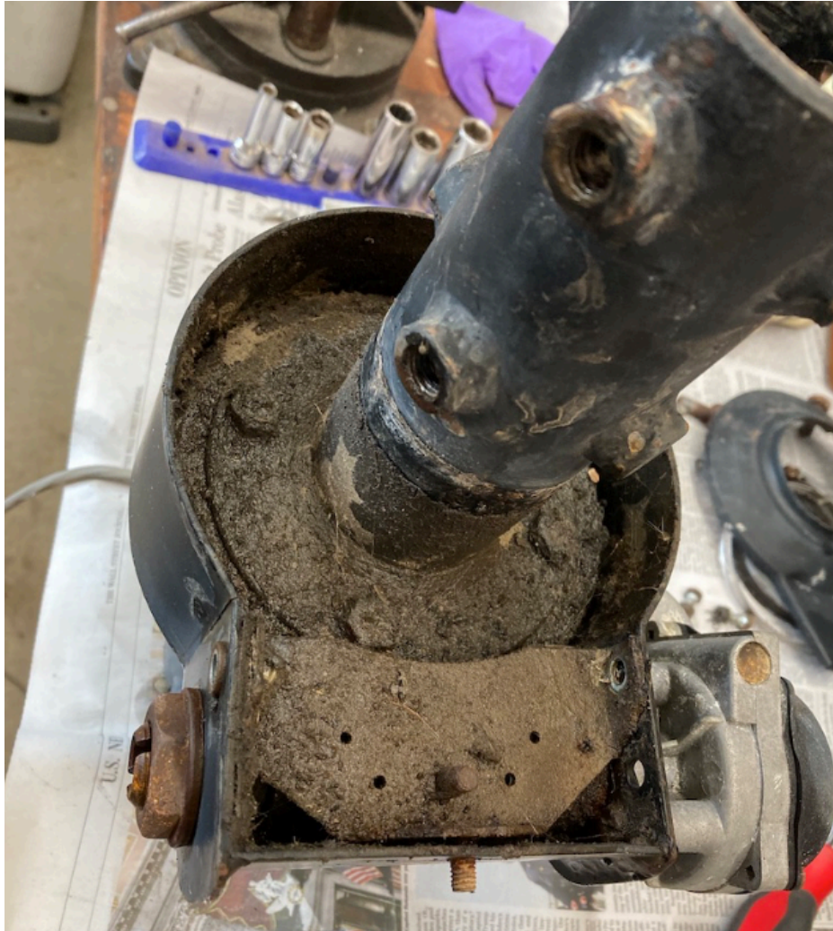
Figure 11. This Alfa-Spid RAK rotator definitely needed servicing.
