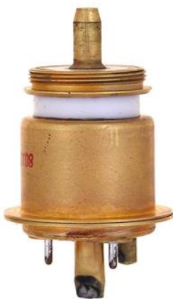
The WE 416 Triode and Amplifier Assembly
