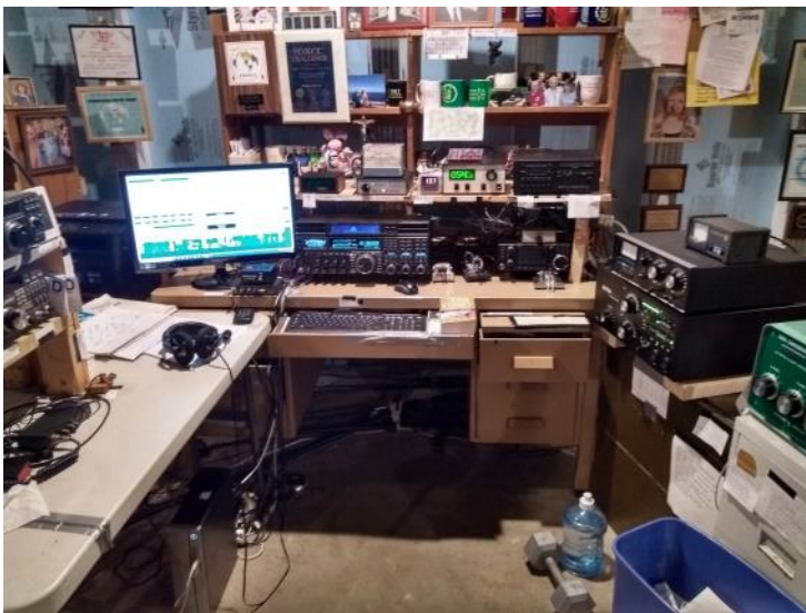
Overall layout of K3MD. Rig on right is backup rig and linear, in case the main rig stops working, and the main backup linear (out of sight on floor) also fails. Backup is essential in radiology, as equipment failure is common.
