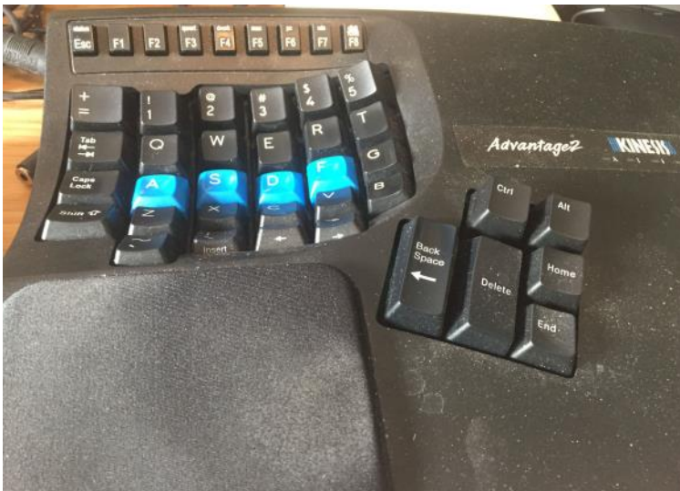
Concave keyboard with common keys moved to thumb.
