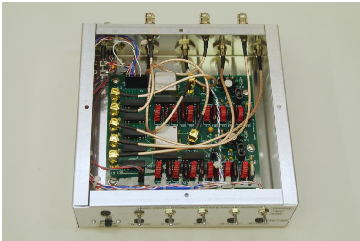
Figure 5. Internal view of the RF distribution box.
