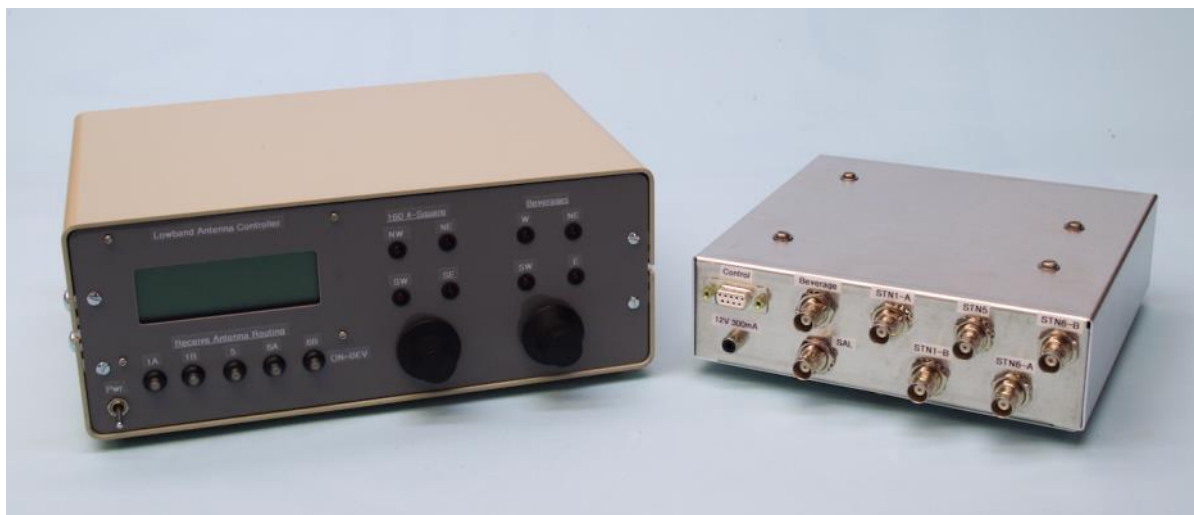
Figure 1. Central controller and RF distribution box.
