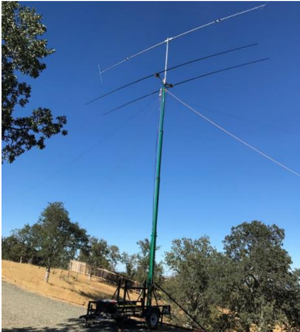
Figure 6. CQP 2019: K6T antennas: 2-el SteppIR at 40ft, 40m Dipole at 50ft, 80m CW Inv-Vee at 37ft.
