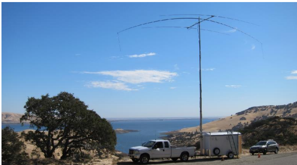
Figure 4. CQP 2019: KU6W antennas: 2-el 20m Yagi, 40m Dipole used on 15m&40m. Antennas at about 40-45ft.
