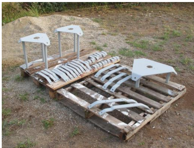
Left: New, painted tower sections Right: Tower top plates and guy brackets
