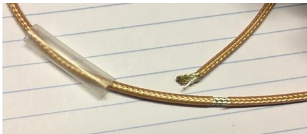
Fig. 6. Ready to solder the loop closed. Heatshrink is in position.
