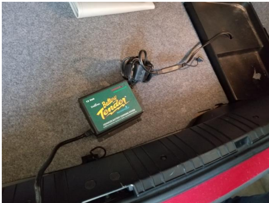
This is a picture of the tender with the installed ferrite core:
