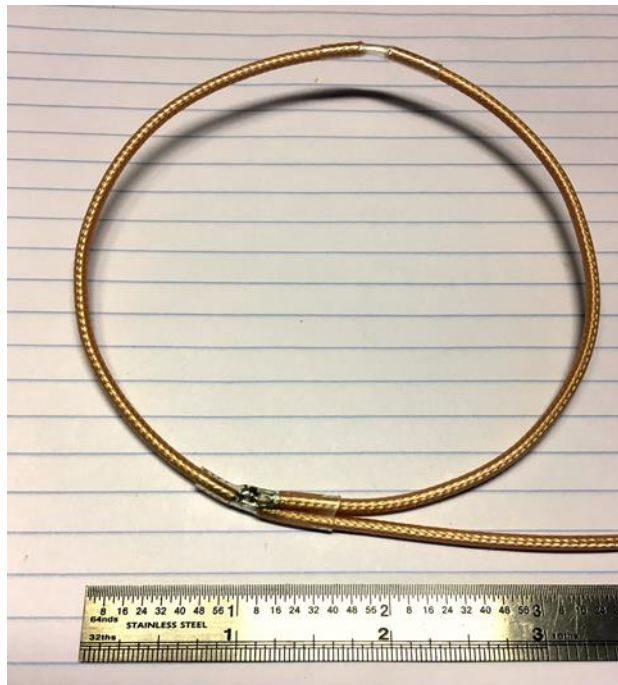
Fig. 7. Completed pickup loop, about 3 inches diameter.
