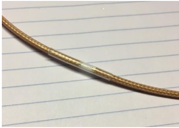
Fig. 5. Midpoint gap in the shield is covered with heatshrink.
