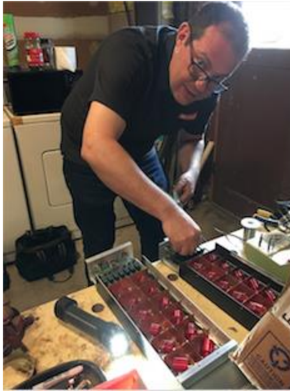
AI6JZ configures bandpass filters.
