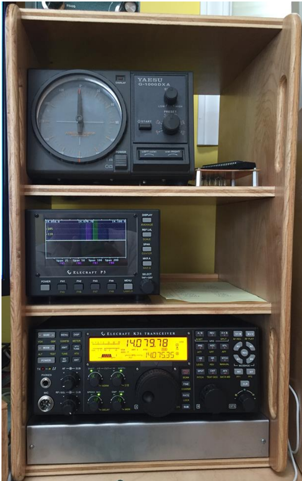
Right (Yellow coded) station - K3S with P3. The Rotor is ready for the new tower to arrive!
