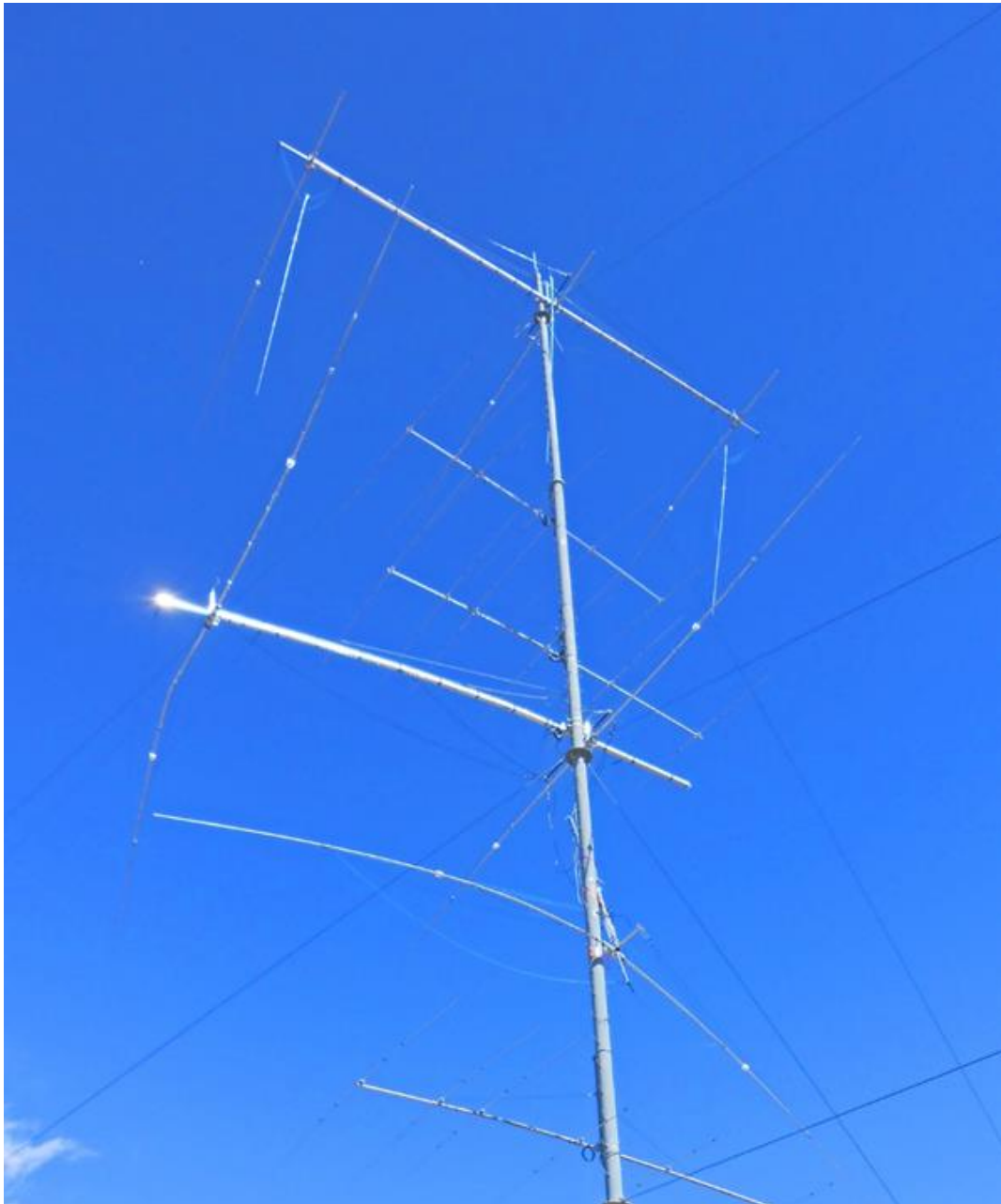
Figure 2 – Elements broken on both 80's. Boom broken on bottom 80.
