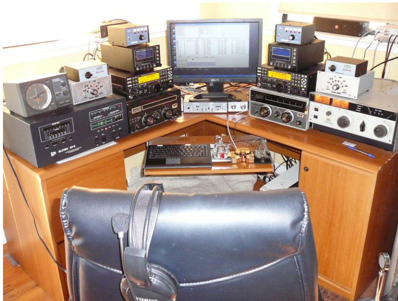
Before: note the Ten Tec tuners underneath both K3s, plus the two RCS-4 controllers atop each P3.
