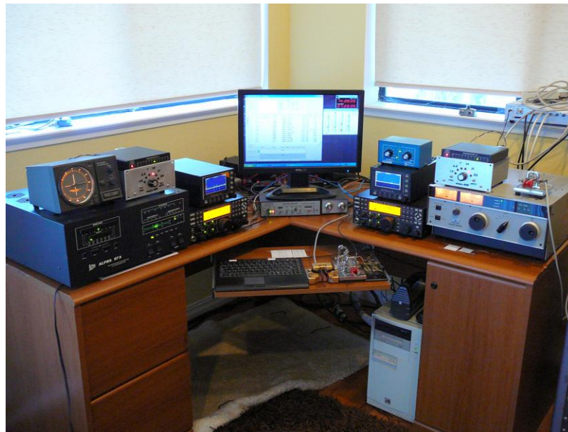
After: No more Ten Tec tuners, slimmer band decoders atop the two ICE 419 boxes, and just one antenna controller atop the right-hand P3.
