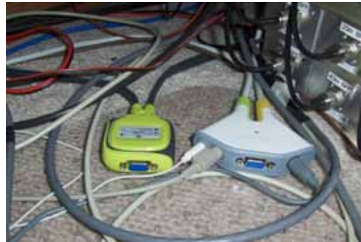
Two models of KVM switches: left one uses double Scroll key presses, right one uses small push button.
